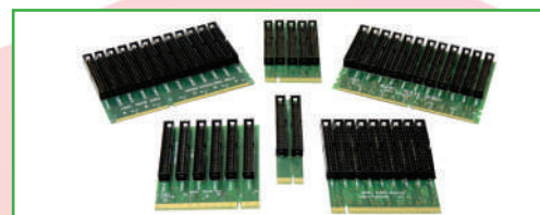
Kit PC, para teste motherboards. Slot's: DDR3, DDR2, PCI, PCIEX1, PCIEX8, PCIEX16.
