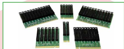
*Kit PC, para teste motherboards. Slot's: DDR3, DDR2, PCI, PCIEX1, PCIEX8, PCIEX16.*
